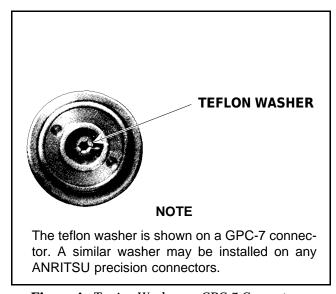
**Figure 4.** Tuning Washer on GPC-7 Connector
