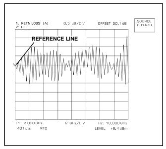
**Figure 8.** Signal Aligned With the Reference Line
