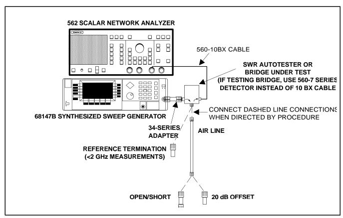
Figure 5. Test Equipment Setup for Directivity Measurement
