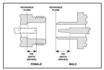
Figure 2. N Connector Pin Depth Definition
