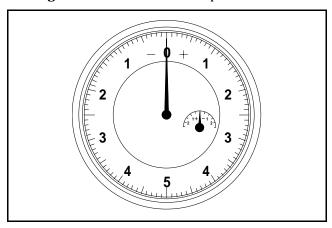
Figure 3. Pin Depth Gauge
