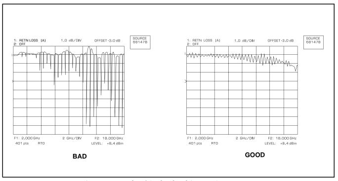
Figure 6. Examples of Good and Bad Air Line Connections
